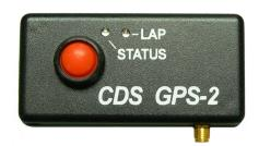
You can use some of the supplied dual-lock material to mount the controller, or use silicone or double sided tape. DO NOT remove the cover or drill holes in the controller box.
